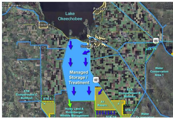
Figure 2 SFWMD Diagram of additional EAA lands needed for more storage, treatment, and conveyance
