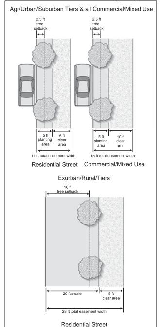
Figure 3.F.2.A-13 - TDD - Sidewalk/Pathway Design Standards
