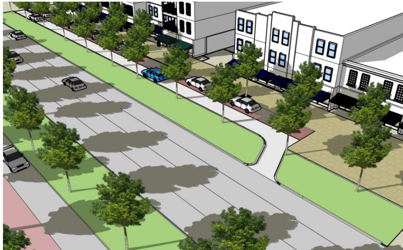
FIGURE 3.B.17.F – TYPICAL EXAMPLE OF SLIP STREET FRONTAGE
