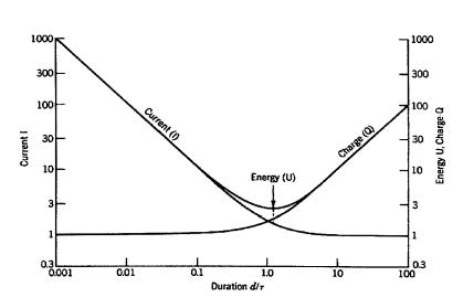
**Figure 1.** Normalized analytical strength-duration curve for current *I*, charge *Q*, and energy *U*. The *x* axis shows the normalized duration of  $d/\tau$ . Note that for  $d \ll \tau$ , *Q* is constant and the most appropriate variable for estimating cell excitation. (from Geddes and Baker, 1989).
