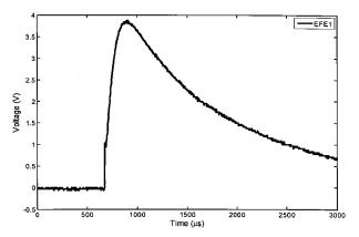
**Figure 4.** Output voltage waveform for EFE1. The maximal charge that flows through the cardiac cell model is given by  $Q = CV = 200 \ \mu\text{F} \times 3.88 \ \text{V} = 775 \ \mu\text{C}$ , the current during which the capacitor charges to maximal value is given by  $I = CV/T = (200 \ \mu\text{F} \times 3.88 \ \text{V})/233 \ \mu\text{s} = 3.33 \ \text{A}$ .
