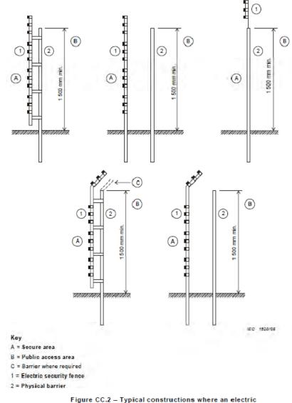
Figure CC.2 – Typical constructions where an electri security fence is exposed to the public
