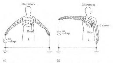
Figure 3 Effect of entry points on current distribution. (a) *Macroshock*, externally applied current spreads throughout the body, (b) *Microshock*, all the current applied through an intracardiac catheter flows through the heart. From F. J. Weibell, "Electrical Safety in the Hospital," *Annals of Biomedical Engineering*, 1974, 2, 126–148.
