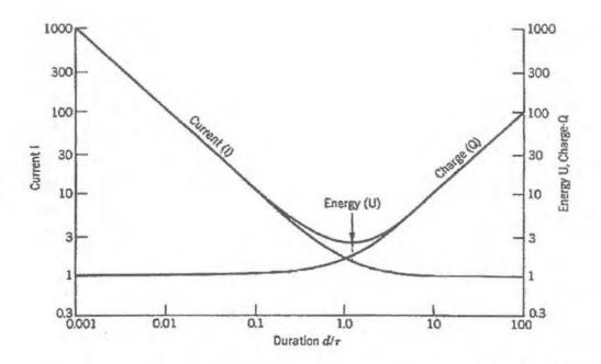
Figure 1. Normalized analytical strength-duration curve for current *I*, charge *Q*, and energy *U*. The x axis shows the normalized duration of  $d/\tau$ . Note that for  $d << \tau$ , *Q* is constant and the most appropriate variable for estimating cell excitation. (from Geddes and Baker, 1989).
