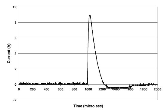
Figure 2. The output current waveform for electric fence energizer with load of 518  $\Omega$ . The output peak current is about 9.0 A.
