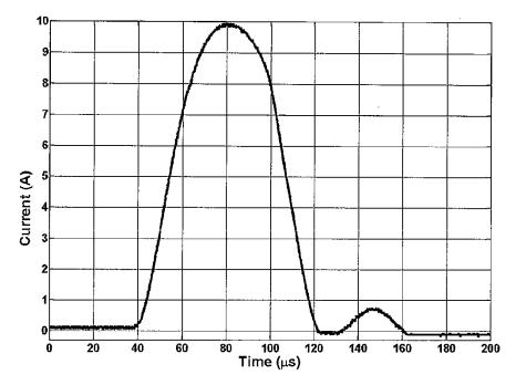
Figure 4. The output current waveform for electric fence controller EFC3. The  $I_{\rm rms}$  according to IEC 60335-2-76 standard for EFC3 is 8.56 A.
