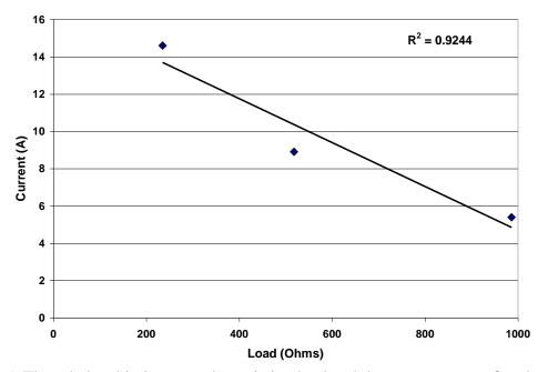
Figure 5. The relationship between the resistive load and the output current for electric fence energizers is linear. The output current drawn from the electric fence energizer increases as the load decreases.
