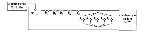
**Figure 1.** The switch S1 is closed to test the EFC according to IEC 60335-2-76 standard. The current flows through a string of 100  $\Omega$  resistors  $R_1-R_5$  (total 498  $\Omega$ ) which approximates the internal body resistance of 500  $\Omega$ . The resistors  $R_6-R_{10}$  in parallel (total 10.09  $\Omega$ ) yields a low voltage that is measured by the oscilloscope.
