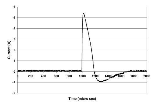
Figure 4. The output current waveform for electric fence energizer with load of 986  $\Omega$ . The output peak current is about 5.4 A.
