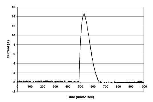
Figure 3. The output current waveform for electric fence energizer with load of 235  $\Omega$ . The output peak current is about 14.6 A.
