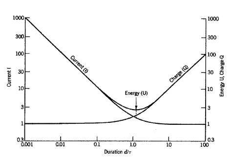
Figure 1. Normalized analytical strength-duration curve for current *I*, charge *Q*, and energy *U*. The x axis shows the normalized duration of  $d/\tau$ . Note that for  $d \ll \tau$ , *Q* is constant and the most appropriate variable for estimating cell excitation. (from Geddes and Baker, 1989).
