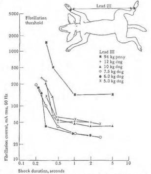
Figure 2 Thresholds for ventricular fibrillation in animals for 60-Hz ac current. Duration of current (0.2 to 5 s) and weight of animal body were varied. Fibrillation current versus shock duration for a 70 kg human is about 100 milliamperes for 5 second shock duration. It increases to about 800 milliamperes for 0.3 second shock duration. From L. A. Geddes, *IEEE Trans. Biomed. Eng.*, 1973, 20, 465–468.
