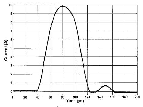
Figure 5. The output current waveform for electric fence controller EFC4. The  $I_{\rm rms}$  according to IEC 60335-2-76 standard for EFC4 is 8.54 A.
