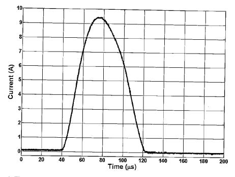
Figure 2. The output current waveform for electric fence controller EFC1. The  $I_{rms}$  according to IEC60335-2-76 standard for EFC1 is 7.89 A.
