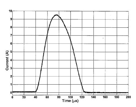
Figure 3. The output current waveform for electric fence controller EFC2. The  $I_{\rm rms}$  according to IEC 60335-2-76 standard for EFC2 is 7.94 A.
