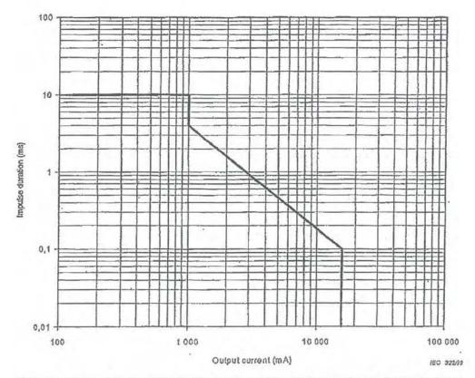
NOTE The equation of the line relating impulse duration (ms) to output current (mA) for 1 000 mA < output current < 15 700 mA, is given by impulse duration =  $41,885 \times 10^3 \times (output current)^{-1,34}$
