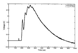
**Figure 5.** Output voltage waveform for the electric fence energizers EFE2. The maximal charge that flows through the cardiac cell model is given by  $Q = CV = 200 \ \mu\text{F} \times 2.91 \ \text{V} = 582 \ \mu\text{C}$ , the current during which the capacitor charges to maximal value is given by  $I = CV/T = (200 \ \mu\text{F} \times 2.91 \ \text{V})/132 \ \mu\text{s} = 4.41 \ \text{A}$ .
