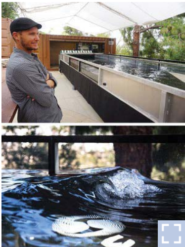
Justin Enjo, an engineer at Wave Loch, "carves water" with a ramp in his experimental wave-making pool near San Diego. So far, the system is able to create tiny, "perfect" surfing waves every 10 seconds.
