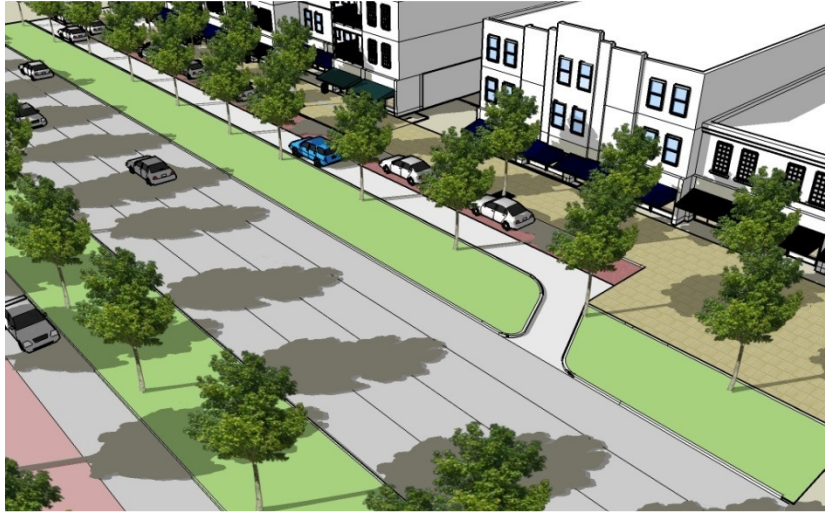
FIGURE 3.B.17.F – TYPICAL EXAMPLE OF SLIP STREET FRONTAGE
