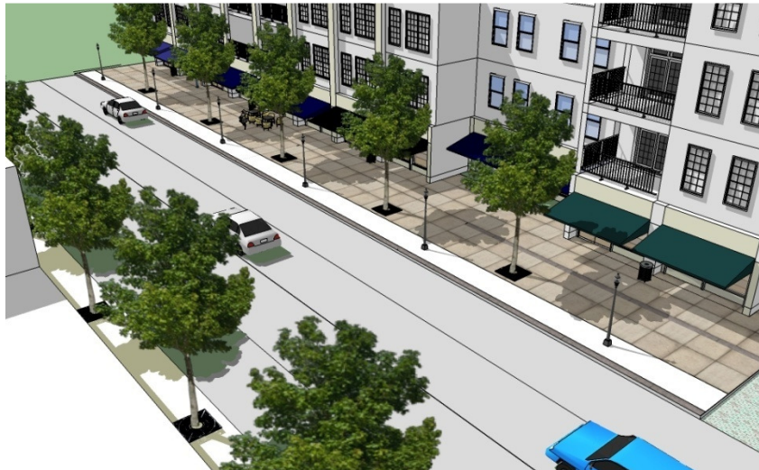
FIGURE 3.B.17.F – TYPICAL EXAMPLE OF PRIMARY FRONTAGE
