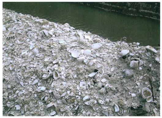
**Figure 3.** Photograph of spoil dredged from a drainage canal located between the West and Northwest Tract. The spoil is from a "shell-rich" naturally deposited marine strata.
