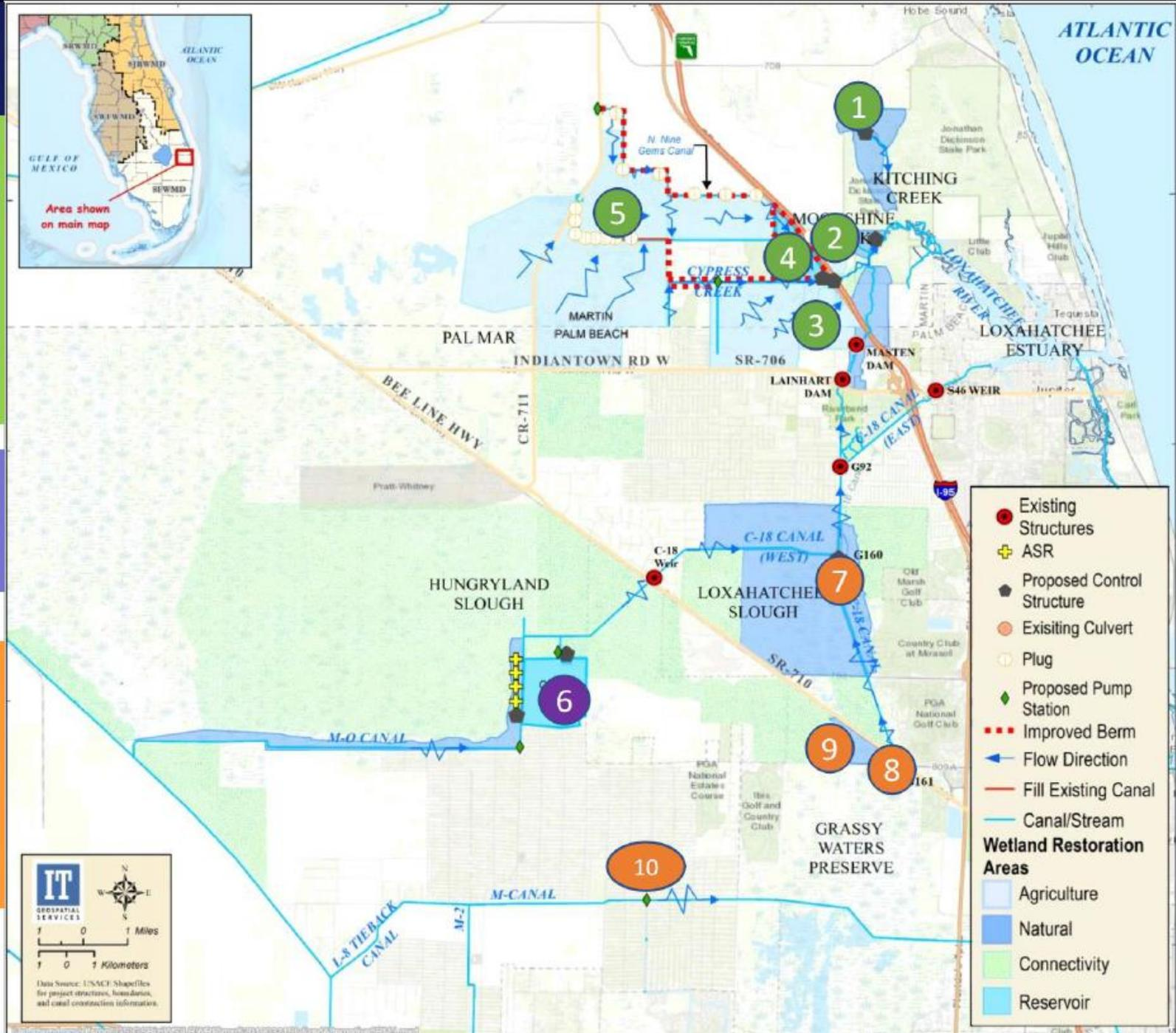
The blue lines show the water routed through GWP (CWPB PS, G-161, G-160, G-92) and the C-18 routes. The orange lines show potential routes that rely on the C-101W Canal.
