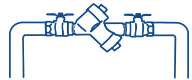
Backflow Prevention Assembly (BFP)
