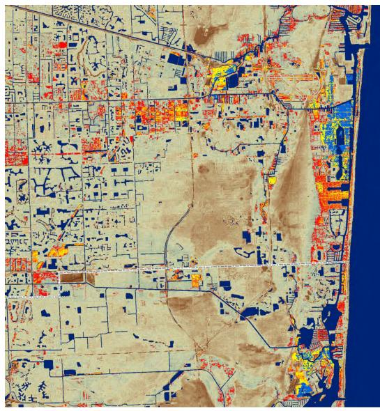
**Figure 15 - SLR Vulnerability at 1 to 3-ft above MHHW (Assuming No Elevation Errors)** Assuming no uncertainty in elevation sources, this figure is an example of analysis output showing areas at an elevation that is at or below MHHW with the following additional feet of water:
