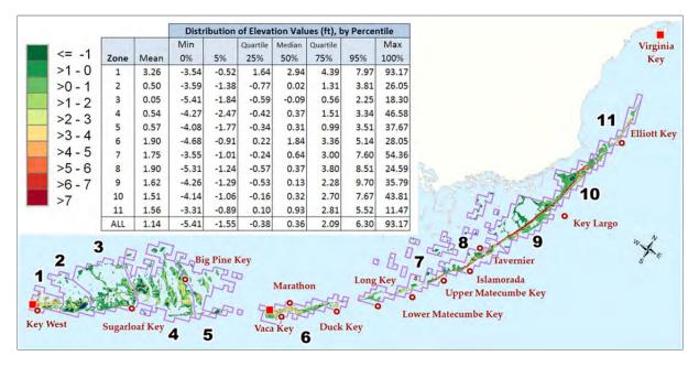
**Figure 3 - Elevation Distribution in the Florida Keys (NAVD88, ft)** The distribution of elevation values was generated using the 25-ft DEM generated from the FDEM LiDAR data. Calculated data is courtesy of Tim Liebermann (SFWMD).
