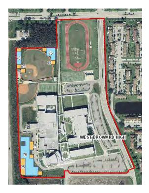
Figure 16: At three foot SLR, the most flooded shelter has only 4.41 acres of inundation, which occurs at the margins of the school grounds.
