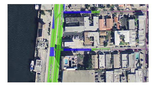
Figure 11: N Ocean Dr doubly digitized. Green represents possible inundation, blue represents more likely inundation. Purple lines are street centerlines. Here, the mileage of N Ocean Dr would be added up twice, once for each side of the road.
