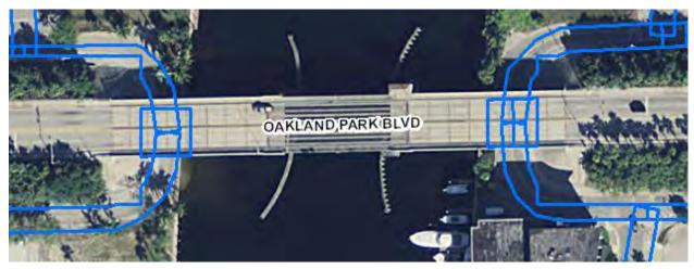
Figure 18: This bridge crosses the Intracoastal Waterway. It appears to have nearby inundation, but the blue, flooded streets shown are actually U-shaped streets under the elevated bridge and do not affect its function.
