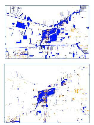
Figure 1: (Top) Inundation grid without water features removed. (Bottom) Inundation grid after water feature removal
