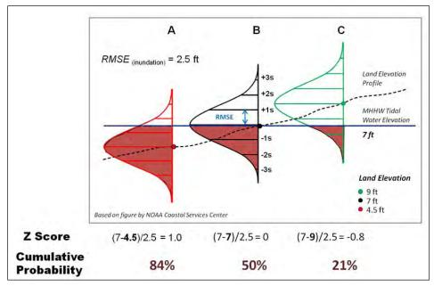
Figure 11 – Z-Score and Cumulative Probability Calculation Example
