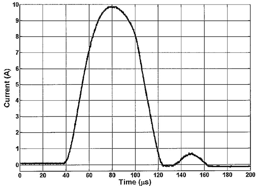
**Figure 5.** The output current waveform for electric fence controller EFC4. The  $I_{rms}$  according to IEC 60335-2-76 standard for EFC4 is 8.54 A.
