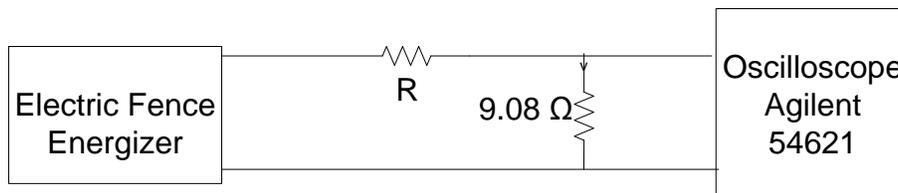
Figure 1. The experimental test set-up to determine the output from electric fence energizer for variable load  $R$ . The current flows through the variable noninductive load  $R$  (235  $\Omega$ , 518  $\Omega$  and 986  $\Omega$ ) which approximates the possible internal body resistances. The 9.08  $\Omega$  yields a low voltage that is measured by the oscilloscope.
