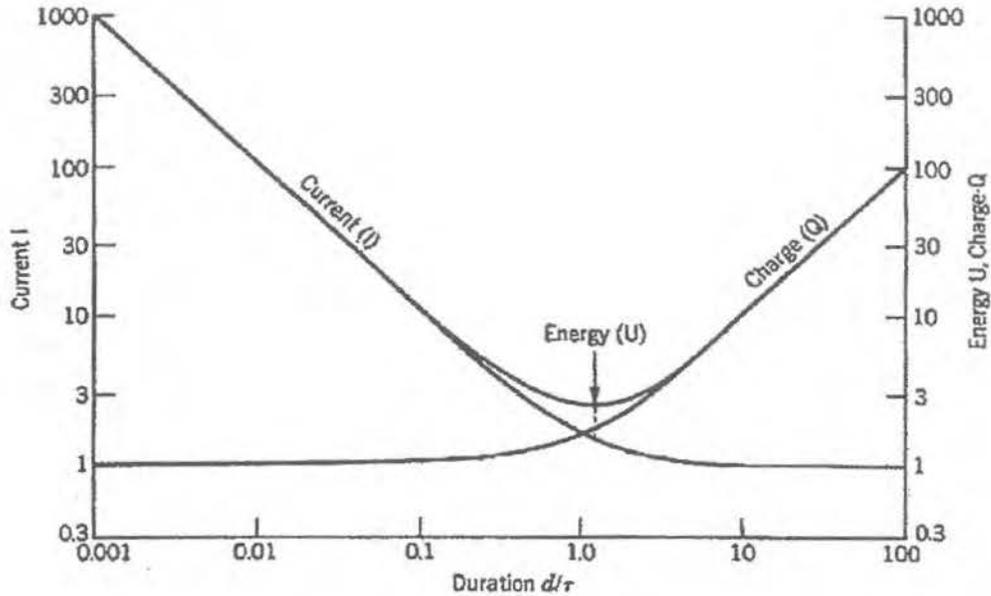
**Figure 1.** Normalized analytical strength-duration curve for current  $I$ , charge  $Q$ , and energy  $U$ . The  $x$  axis shows the normalized duration of  $d/\tau$ . Note that for  $d \ll \tau$ ,  $Q$  is constant and the most appropriate variable for estimating cell excitation. (from Geddes and Baker, 1989).
