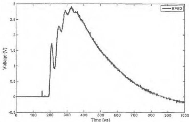
**Figure 5.** Output voltage waveform for the electric fence energizers EFE2. The maximal charge that flows through the cardiac cell model is given by  $Q = CV = 200 \mu\text{F} \times 2.91 \text{ V} = 582 \mu\text{C}$ , the current during which the capacitor charges to maximal value is given by  $I = CV/T = (200 \mu\text{F} \times 2.91 \text{ V})/132 \mu\text{s} = 4.41 \text{ A}$ .
