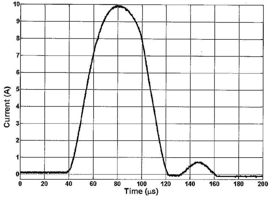
**Figure 4.** The output current waveform for electric fence controller EFC3. The  $I_{rms}$  according to IEC 60335-2-76 standard for EFC3 is 8.56 A.
