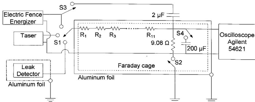
**Figure 2.** The EFE is selected by S1. The current flows through a string of 47  $\Omega$  resistors  $R_1$ – $R_{11}$  (total 518  $\Omega$ ) which approximates the internal body resistance of 500  $\Omega$ . The 9.08  $\Omega$  yields a low voltage that is measured by the oscilloscope.
