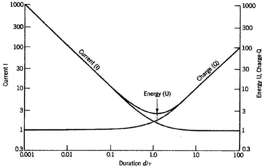
**Figure 1.** Normalized analytical strength-duration curve for current  $I$ , charge  $Q$ , and energy  $U$ . The  $x$  axis shows the normalized duration of  $d/\tau$ . Note that for  $d \ll \tau$ ,  $Q$  is constant and the most appropriate variable for estimating cell excitation. (from Geddes and Baker, 1989).
