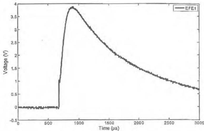
**Figure 4.** Output voltage waveform for EFE1. The maximal charge that flows through the cardiac cell model is given by  $Q = CV = 200 \mu\text{F} \times 3.88 \text{ V} = 775 \mu\text{C}$ , the current during which the capacitor charges to maximal value is given by  $I = CV/T = (200 \mu\text{F} \times 3.88 \text{ V})/233 \mu\text{s} = 3.33 \text{ A}$ .
