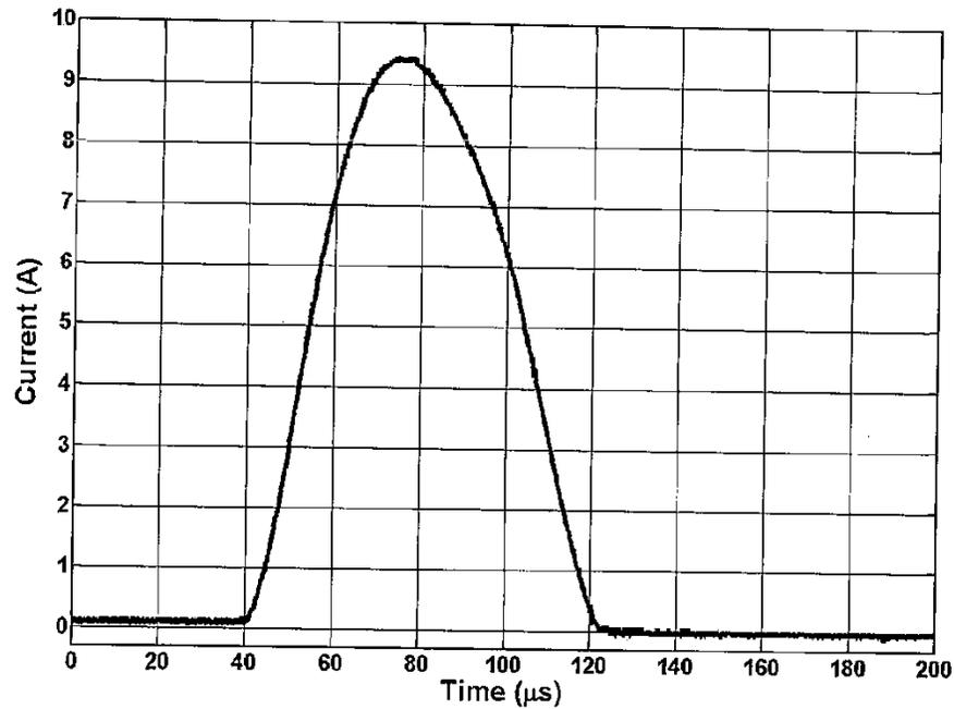
**Figure 2.** The output current waveform for electric fence controller EFC1. The  $I_{\text{rms}}$  according to IEC60335-2-76 standard for EFC1 is 7.89 A.
