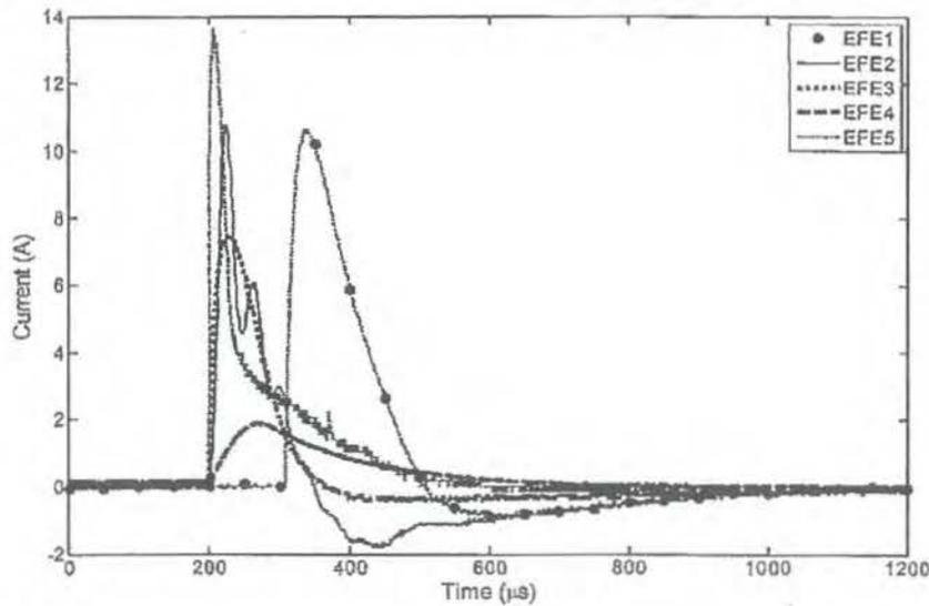
**Figure 3.** The output current waveform for five EFEs. EFE1 yields about 7.75 A for 151  $\mu\text{s}$  = 1170  $\mu\text{C}$ , EFE2 yields about 3.34 A for 345  $\mu\text{s}$  = 1150  $\mu\text{C}$ , EFE3 yields about 5.69 A for 91  $\mu\text{s}$  =
