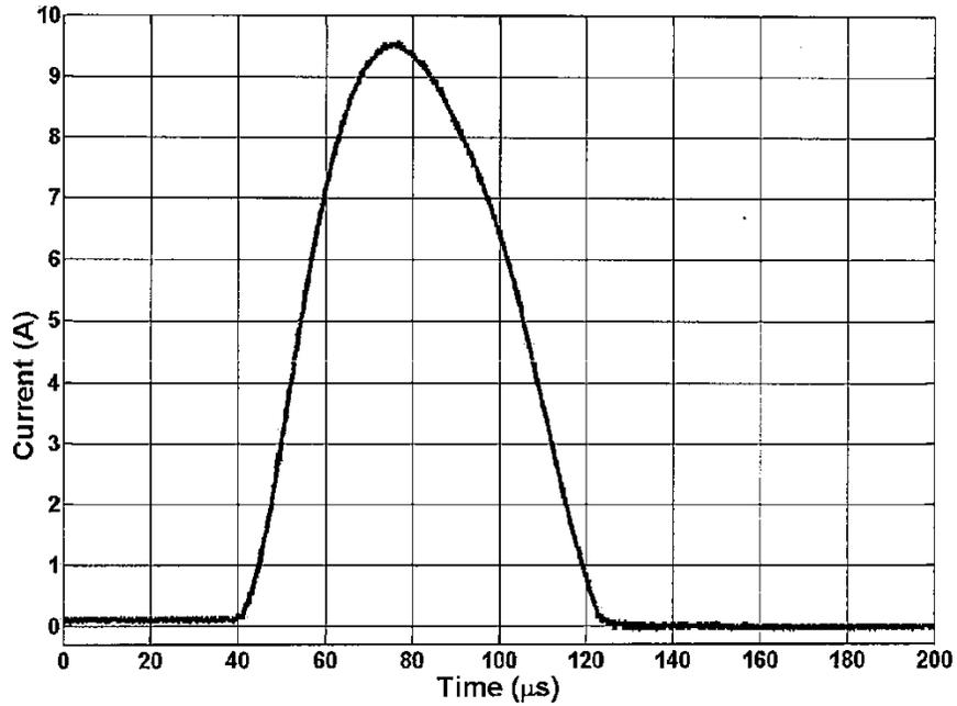
**Figure 3.** The output current waveform for electric fence controller EFC2. The  $I_{rms}$  according to IEC 60335-2-76 standard for EFC2 is 7.94 A.
