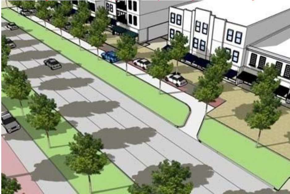
Figure 3.B.16.E – Typical Example of Slip Street Frontage
