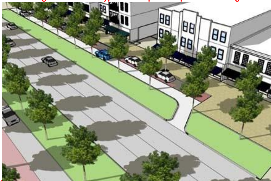
Figure 3.B.16.E – Typical Example of Slip Street Frontage
