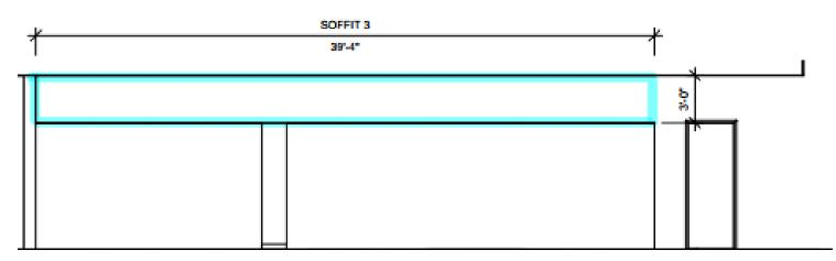
Graphic below illustrates soffit one (1) adjacency to stairwell walls and contiguous placement of soffits.
