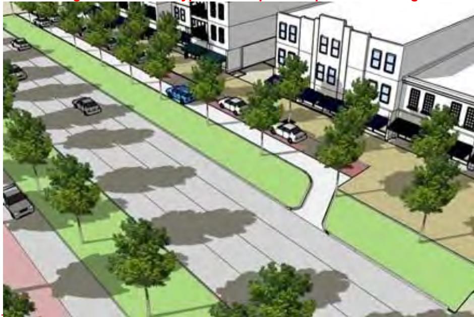
Figure 3.B.16.E – Typical Example of Slip Street Frontage
