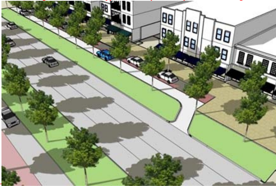
Figure 3.B.16.E – Typical Example of Slip Street Frontage
