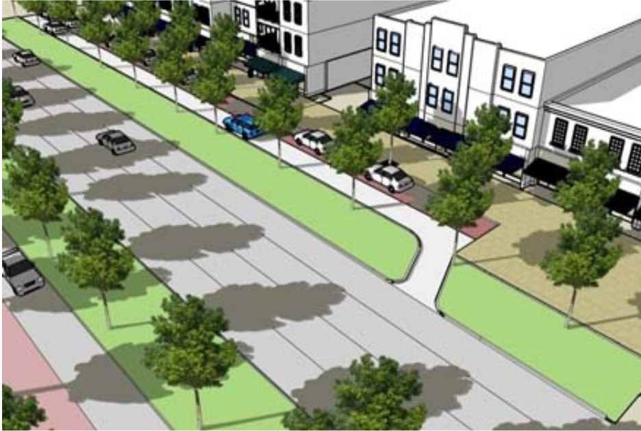
Figure 3.B.16.E – Typical Example of Slip Street Frontage
