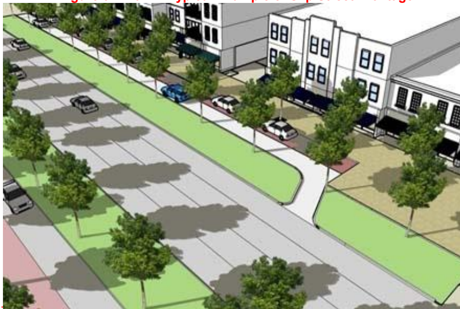
Figure 3.B.16.E – Typical Example of Slip Street Frontage
