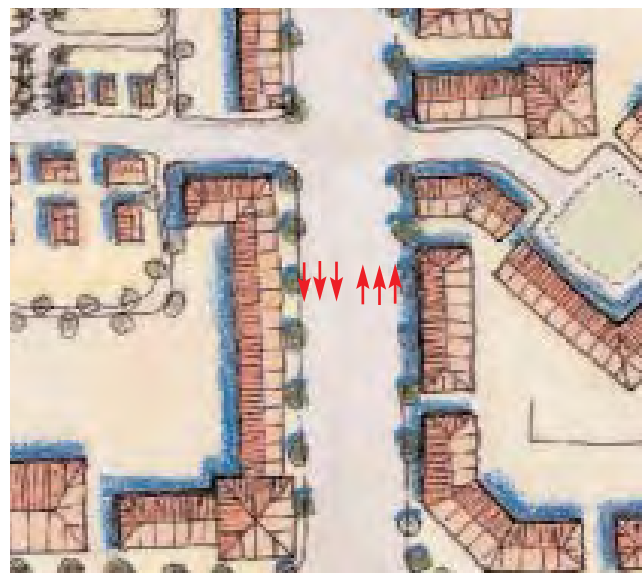
Proposed Changes with new private redevelopment: six 11' travel lanes with right and left turns at main intersections. Lane width reduced over time.
