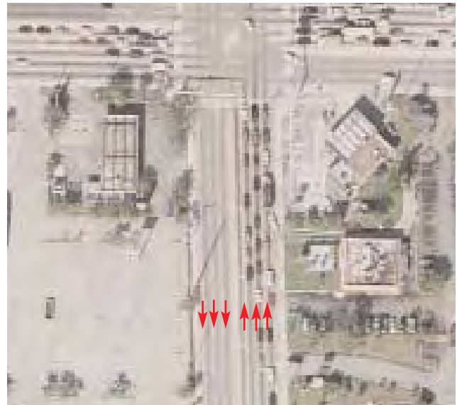
Existing Condition: six 11' travel lanes right and left turn at main intersections.
