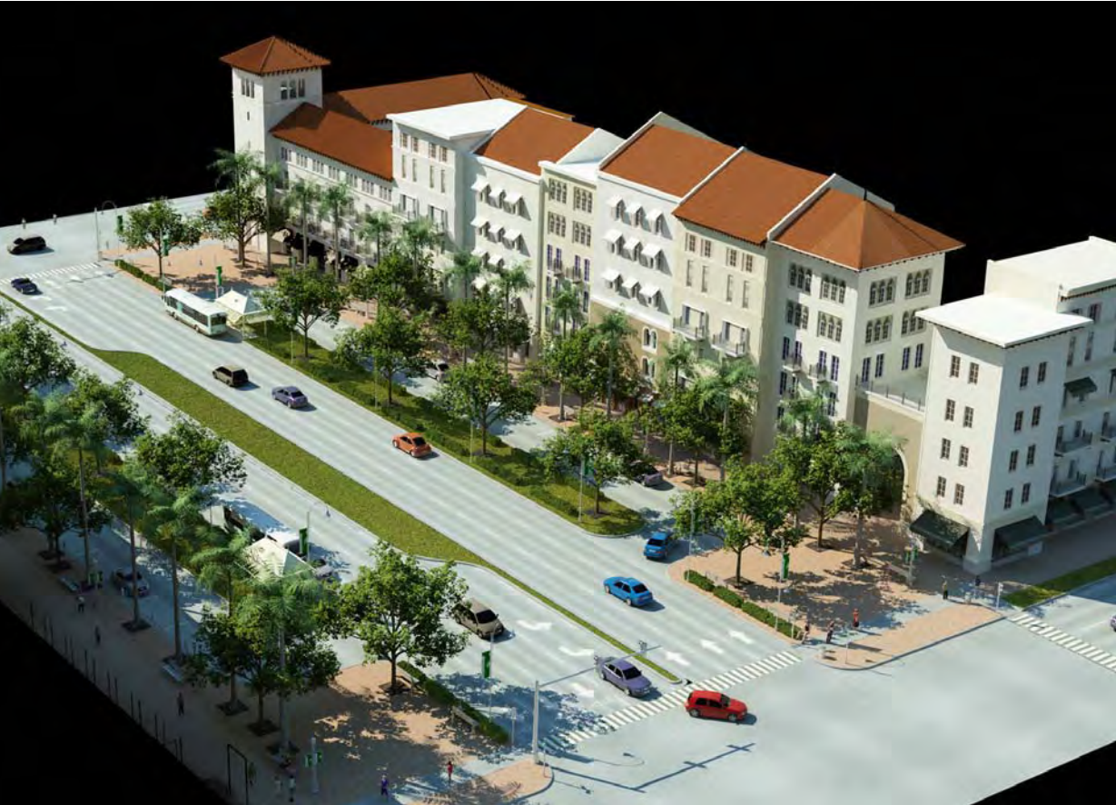
This oblique view shows an idealized Military Trail. At points where there is sufficient real estate, frontage or service roads must be provided for local traffic distribution, for on-street parking that is crucial to commercial vitality, to improve transit potential, and to humanize the corridor. Where dimensionally possible, this technique should be required.
