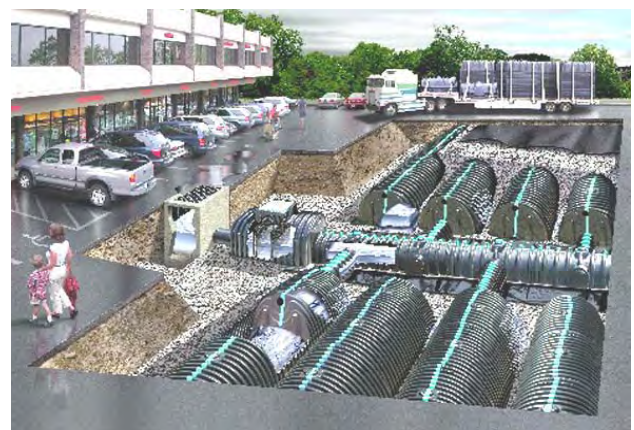
Storm water exfiltration system designed for a parking lot
