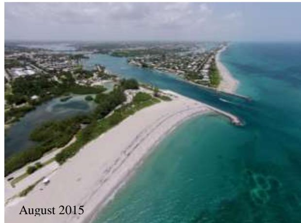
In the late 1960's, a sand trap was dredged approximately 1000 feet west of the inlet mouth, and the jetties were modified. The wing on the seaward end of the south jetty was removed in 1967 in an attempt to reduce shoaling within the inlet. Both jetties were extended landward to prevent flanking. The inlet channel is currently 195 feet wide and 6 feet deep (Mehta, Montague, and Parchure 1990).
