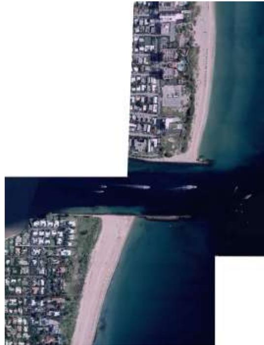
Following a feasibility study, a sand transfer plant was installed on the north side of the north jetty in 1957-58 at a total cost of \$544,539. The facility began operation in August 1958, pumping sand south across the inlet and depositing it on the downdrift beach.
