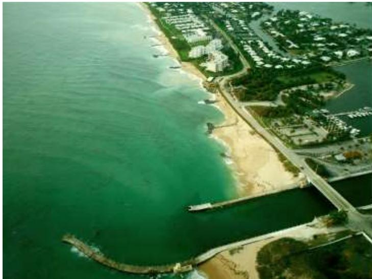
In 2001, the county removed a rock ledge within the throat of the inlet and created a sand trap behind the training wall. The County conducted maintenance dredging of the sand trap, a portion of the ICW, and the Boynton Boat Club Channel in 2001, 2008, and 2013. Dredged sand was discharged south of the inlet near Ocean Hammock Park and elsewhere in the ICW.
