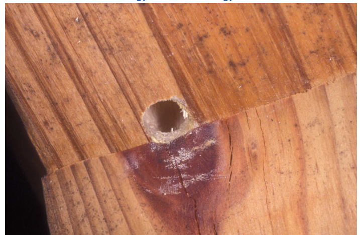
Figure 4. Carpenter bee damage to mailbox.
