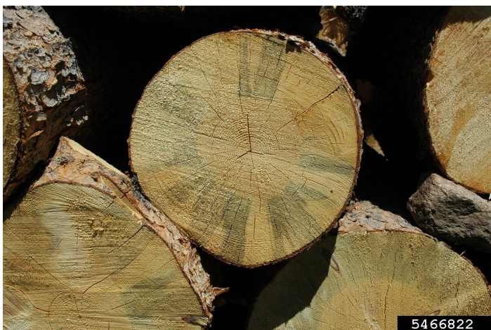
Figure 2. Pine logs discolored by blue stain fungus transmitted by pine beetle.
